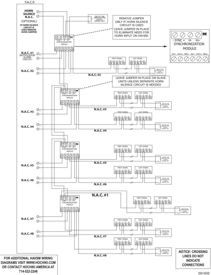
A WARNING The master control module must be powered at the same time or prior to the slave modules for proper operation.
